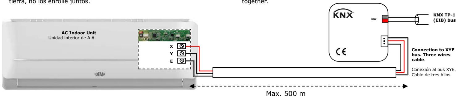
**IMPORTANT:** If the INKNXMID\*\*\*I000 gateway is **not** placed at one end of the XYE bus, the terminal resistor should be deactivated. Remove Jumper 1 to deactivate the 120 Ω terminal resistor.
